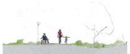
Timber boardwalk with in-built seating and solar lighting. Clean links between path structure and adjacent natural areas
